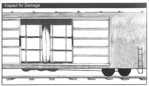
Producers make every effort to block loads securely with either timbers, dunnage boards or airbags. The illustration above shows when an airbag is used to transport units of panels by railcar.
